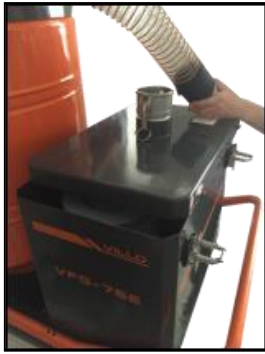
Fig. 4.5 cartridge filter cleaning
