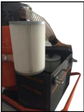
Fig. 4.6 cartridge filter cleaning
