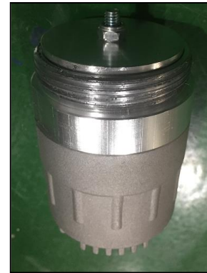
Fig. 3.6 Pressure Control Valve
