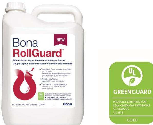
Bona RollGuard is a single-component, rollable silane-based sealer designed to reduce vapour transmission from subfloors with high residual moisture content. It is suitable for conforming green concrete substrates with up to 95% relative humidity. Bona RollGuard delivers reliable, long-lasting performance and is fully compatible with all Bona silane-based adhesives.
